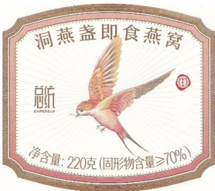
The label central image of a Golden Swiftlet is printed in four colour process, using a particularly fine screen ruling, but in excellent register. The image is further highlighted by the use of very accurate embossing emphasising the feathers.
